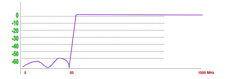
This High Pass Filter is often installed at all the customer premise, where no Cablemodem service is required. This help keep the return system free of Ingress, coming from customer.
