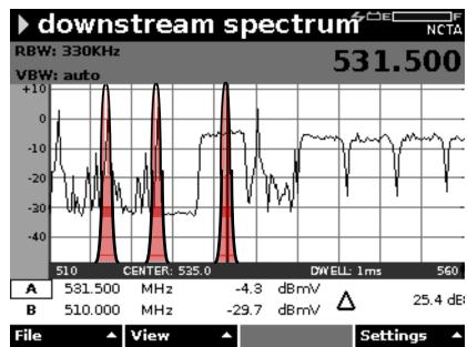
Analog and digital (broadcast) QAM signal. The recommended delta in level should be 6 to 10 dB.
