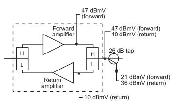
Figure A-2 illustrates a section of the plant where forward path levels are *lowered* to 43 dBmV with the subsequent selection of a lower value tap. When a constant tap port injection level is maintained, the level will be 4 dB too high at the diplex filter. To compensate, the return path level should be aligned 4 dB higher at this station by one of the following methods:
