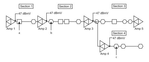
Figure 2.3 indicates that, at the highest channel, the output level is +47 dB at each amplifier station. Because all stations are set to the same level, the gain from one station's output to the next station's output is 0 dB, or "unity" gain. During forward path setup, the gain of each station is adjusted so that it exactly matches the loss of the cable and passives that preceded it.
