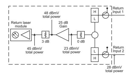
Figure 2.2 identifies two levels that are significant: (1) the return path input level at the station port (28 dBmV) and (2) the level at the laser module or transmitter (45 dBmV). The difference between these levels is the node return gain. In this example, the required node return gain is 45 - 28 = 17 dB. These two absolute levels (input and transmitter) will probably not be used in the setup process, but the node return gain will be used. This example shows
