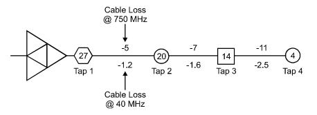
Table 2.3 shows the resulting loss of the feeder cable and taps between the amplifier and the tap port for both the forward and return paths:
