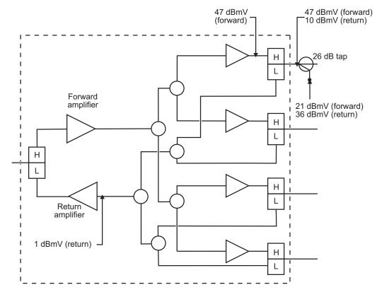
Figure 2.4 and Figure 2.5 show a signal being injected into a 26 dB tap that is connected to the station's output port (see *note* below). In both cases, the injected signal is 36 dBmV at the tap port. After passing through the 26 dB loss of the tap, both signals arrive at the diplex filter at 10 dBmV. Because a constant level is required at every output diplex filter, the plant is properly aligned. In other words, 36 dBmV is required at a 26 dB tap, regardless of the amplifier type.
