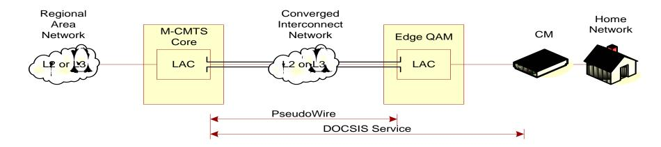
DEPI is based upon a L2TPv3 (RFC 3931) pseudowire that exists in the downstream direction between a DOCSIS MAC in a M-CMTS Core and a DOCSIS PHY in an EQAM.
