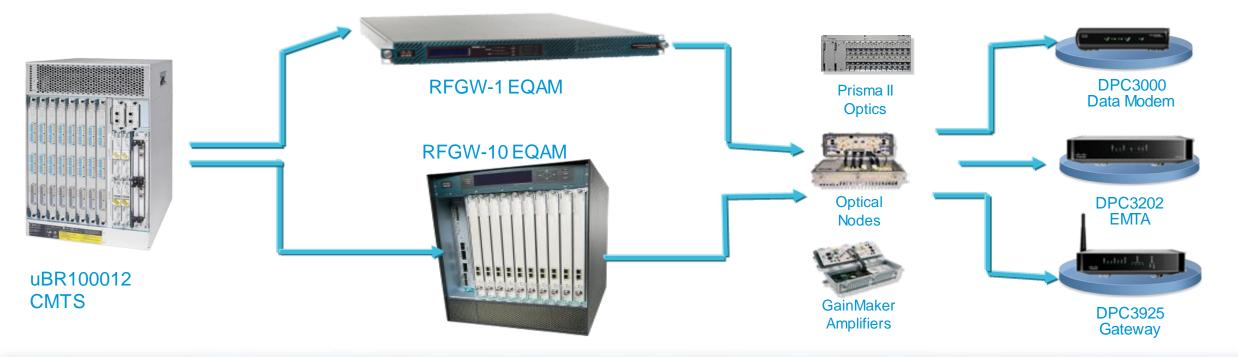
• M-CMTS architecture allows use of Universal Edge QAM supporting both DOCSIS and Video services to maximize QAM channels per port
