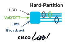
Different sets of downstream channels, one or several bonding group Unused bandwidth from one service cannot be used by another service
