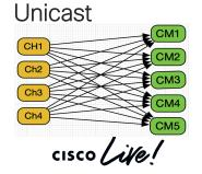
Personalized linear TV and VoD delivered to each subscriber Highest CMTS DS capacity/cost and spectrum requirements Alleviates multicast requirements on end-to-end IP Video system
