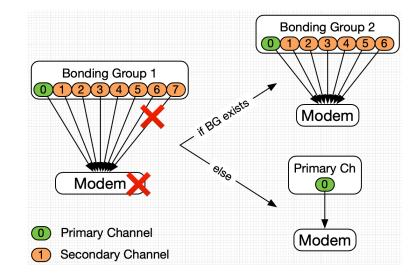
Multicast running over available RF(s) after modem reload
